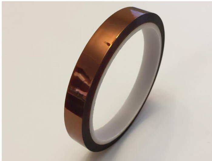
Figure 22: Example of the low static Kapton tape
