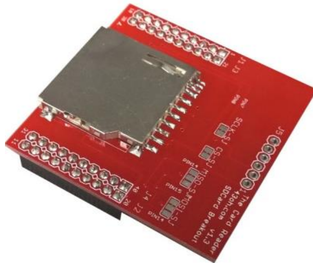
Figure 37: SD card BoosterPack for the Launchpad that is available from 43oh.com (reprinted with permission from 43oh.com)
