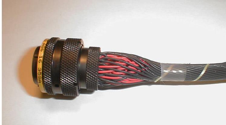
Figure 30: Example of concentric twisting and service loops (reprinted with permission from RB Racing)
