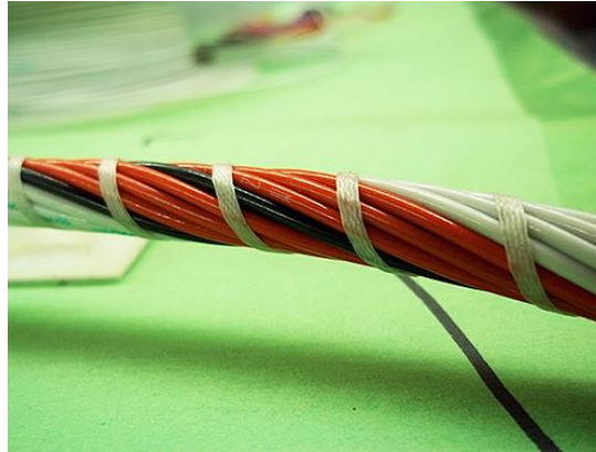
Figure 33: Example of concentrically twisted and laced section of wiring harness (reprinted with permission from RB Racing)
