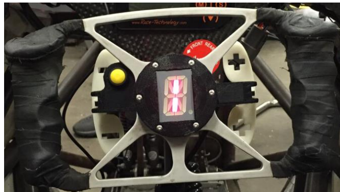
Figure 10: Actual photo of steering wheel with display and driver controls
