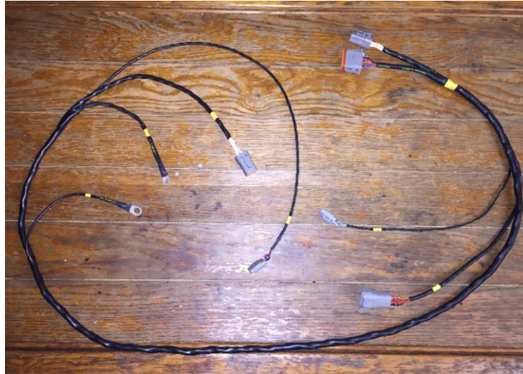
Figure 42: Actual photo of completed wiring harness
