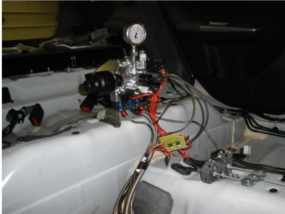
Figure 8: setup of hydraulic shifting system (awaiting permission from sssdrive to reprint)
