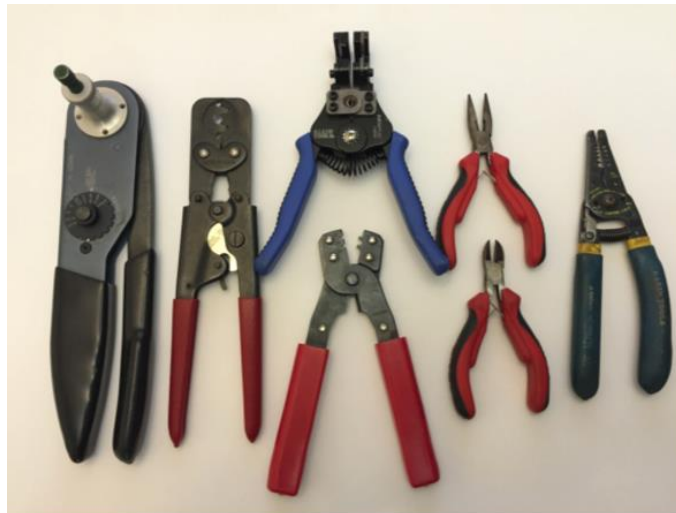
Figure 24: Example of some of the necessary tools to build wiring harnesses
