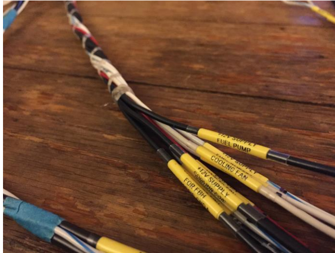
Figure 27: Example of labels with clear heat-shrink on each wire
