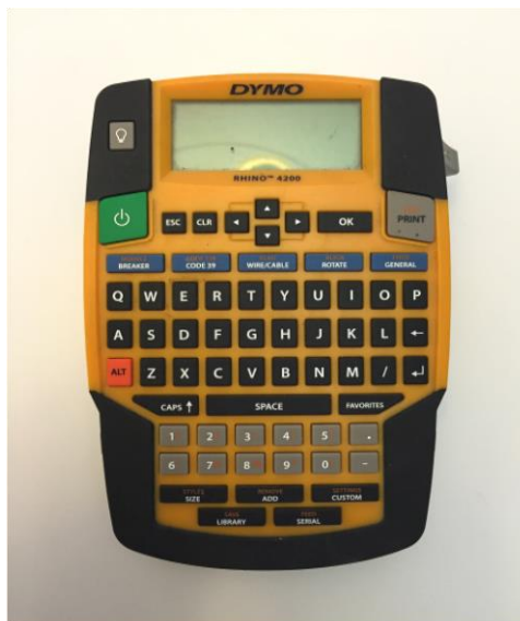
Figure 26: Example of a label maker capable of printing wire labels
