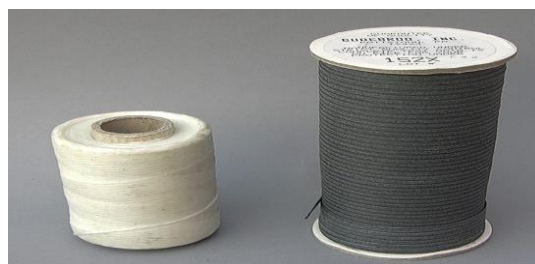
Figure 23: Example of Kevlar braided lacing cord (reprinted with permission from RB Racing)
